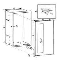
\*NOTE: THE ABOVE DIMENSIONS ARE FOR NON FIRE-RATED CABINETS, ROUGH OPENING DIMENSIONS AS WELL AS OUTSIDE FLANGE AND DOOR DIMENSIONS ARE LARGER FOR FIRE-RATED OCCULT CABINETS - SEE FIRE-RATED OCCULT SERIES.
